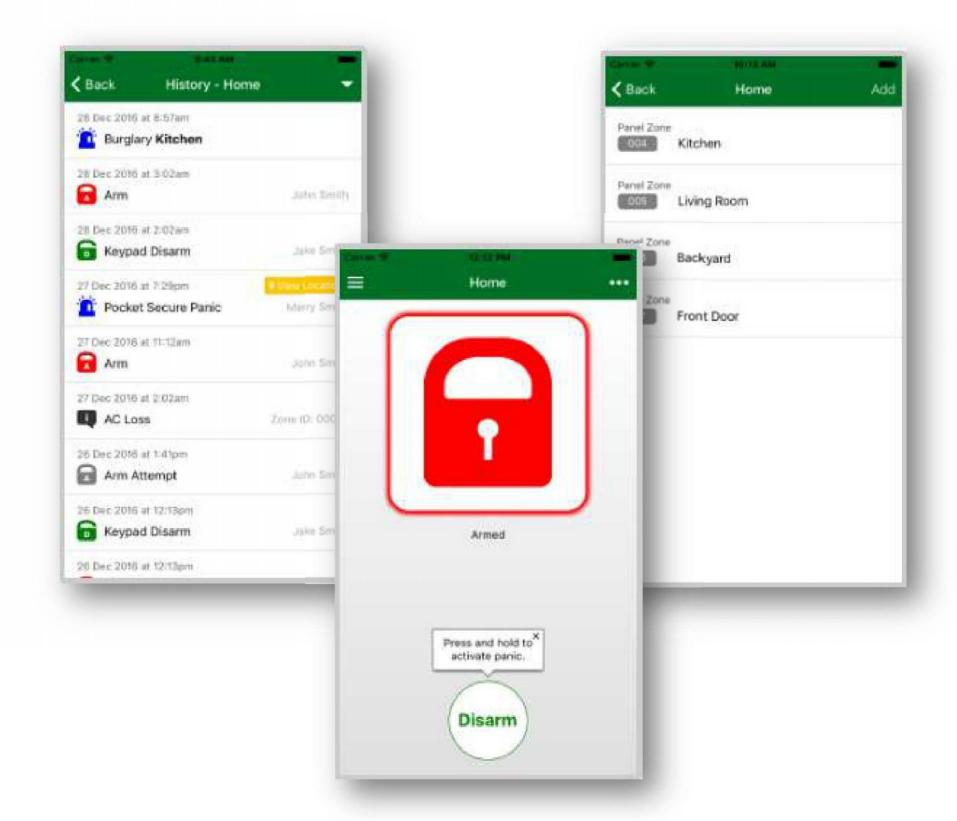
To toggle the state of the alarm, the app presents an interface to pulse output 1 on the **SafeDial Wireless** unit in the field. This then forces the app to wait until the next open/close event is sent and updates the app with the new state.
